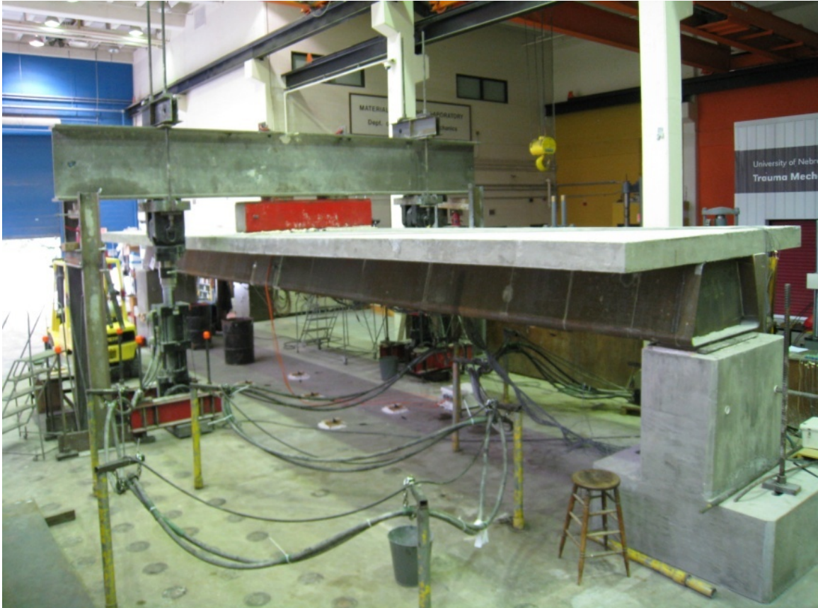
FIGURE 2-18: COMPOSITE TEST SETUP
