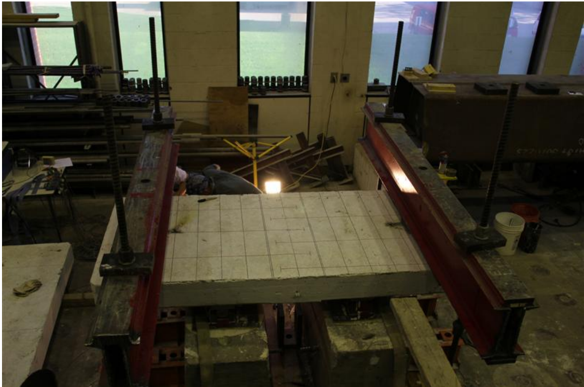
FIGURE 6-11: SLAB TEST SETUP
