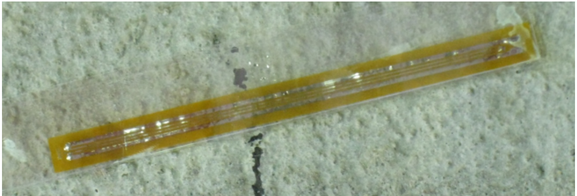
FIGURE 2-15: TYPICAL CONCRETE SURFACE GAGE USED DURING TESTING
